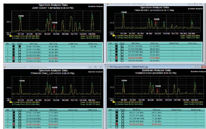
Scanning for Interference on FM Broadcasting Channels
